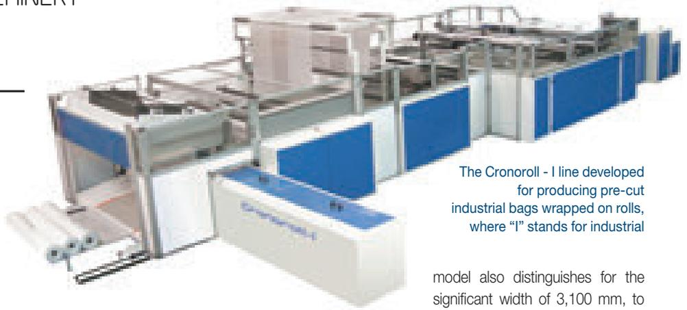
The Cronoroll - I line developed for producing pre-cut industrial bags wrapped on rolls, where "I" stands for industrial
