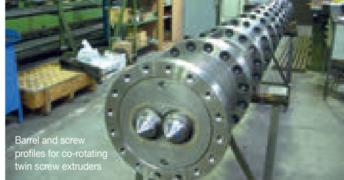
Barrel and screw profiles for co-rotating twin screw extruders
