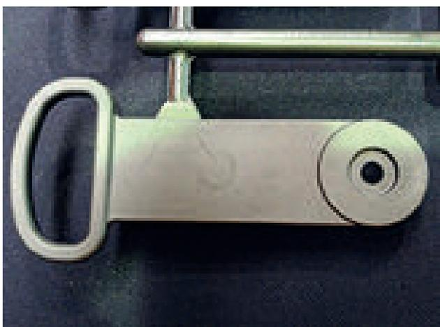
Fig. 1 - Circular marks on an injection moulded piece
