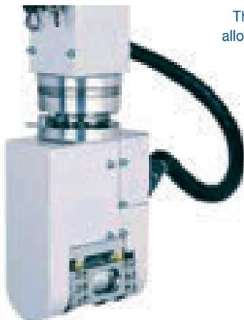
The servo head option consists of two additional AC servomotors which allow rotation around the vertical axis and around the product overturning axis. Operating range: A = 0-188° and rotation around C axis = 0-320°
