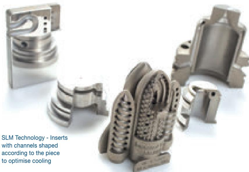
SLM Technology - Inserts with channels shaped according to the piece to optimise cooling
