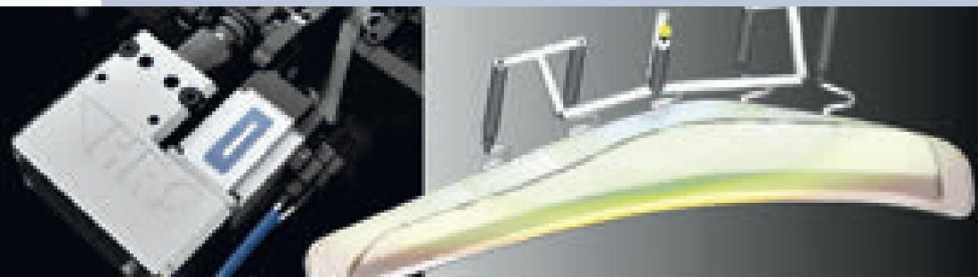
Servo-drive for the FlexFlow system for precise regulation of the hot runner nozzle valve (left in the photo), developed for a sequential mould with 5 injection points for the production of large PC crystal lenses for car headlights (on the right in the photo)
