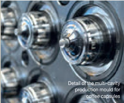
Detail of the multi-cavity production mould for coffee capsules
