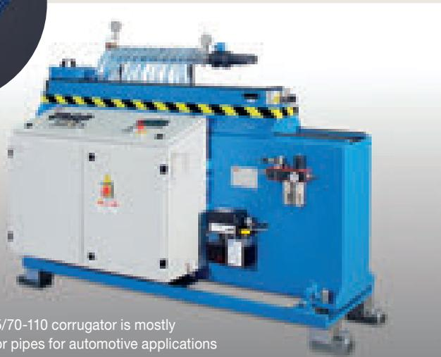
The FMV15/70-110 corrugator is mostly intended for pipes for automotive applications
