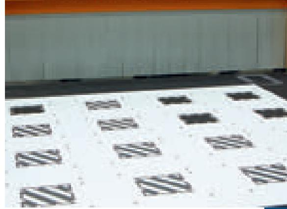
Sheet machining using a Skill Plast FT 1224
