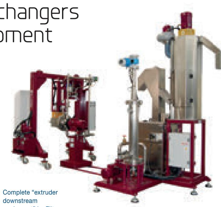
Complete "extruder downstream equipment" by Filtec
