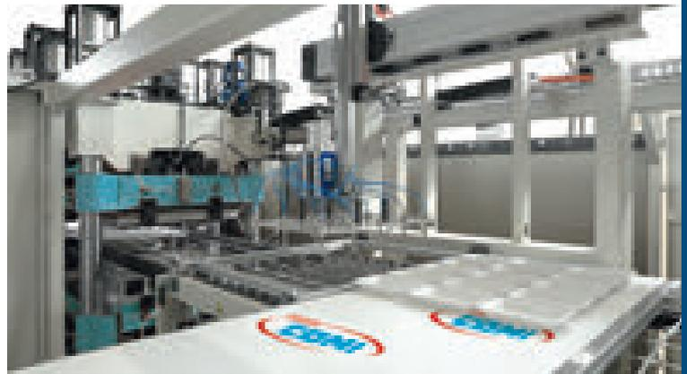
machines is completely servodriven and equipped with a new software for cycle control that, along with a user friendly HMI, guides the operator through the setting pages, providing full diagnostic analysis.
