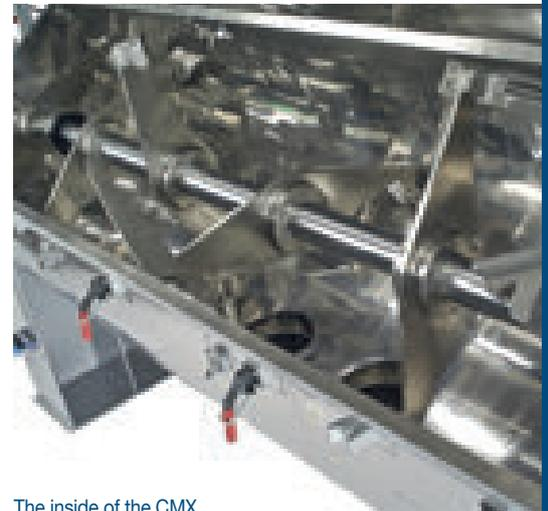
The inside of the CMX high efficiency horizontal cooler
