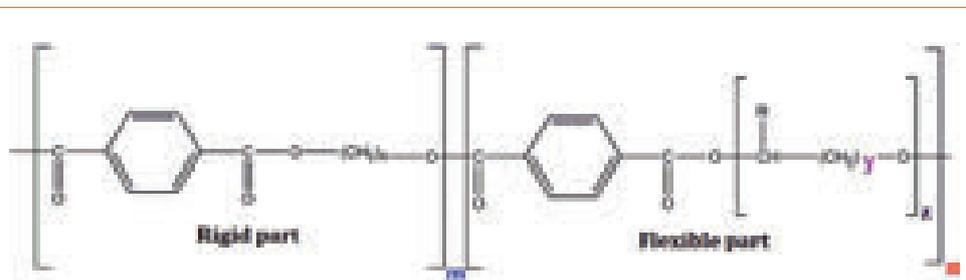
Fig. 1 - The macromolecular structure of Sipolprene thermoplastic ether ester elastomers (TPC-ET)
