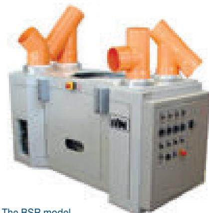
The BSR model is a semiautomatic belling machine for short pipes up to two metres long
