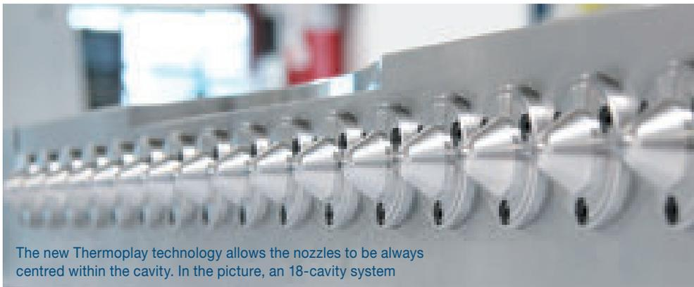
The new Thermoplay technology allows the nozzles to be always centred within the cavity. In the picture, an 18-cavity system
