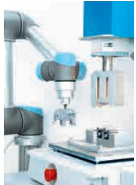
VDMA Blue Competence concept study for Fakuma 2014: standard modular ultrasonic welder HiQ Dialog with small-scale robot: handling, testing, welding, and marking of a toy elephant
