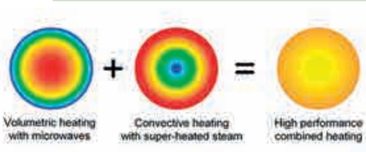
Working principle of combined drying MW-SHS (microwave and super-heated steam) for hygroscopic polymers
