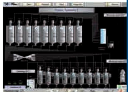
Screen for the supervision system, material storage, drying and centralised feeding
