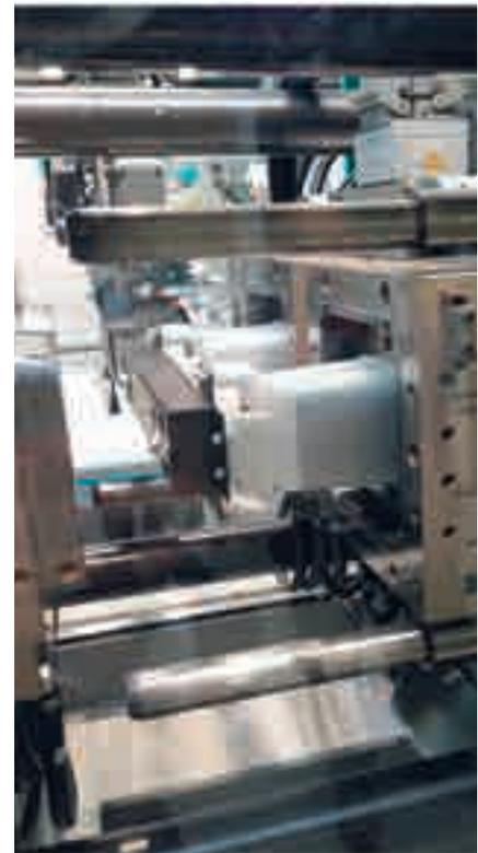
The application developed in cooperation with Arburg and Hofstetter underlines the attention towards the mould open time, and thus to total cycle time
