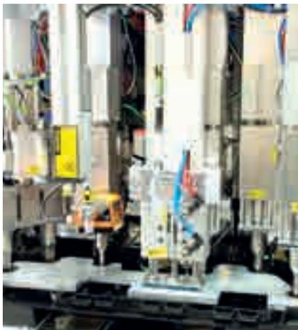
Fig. 1a - Function integration in multi-head welding machine for automobile engine cover: entire tool change kit
