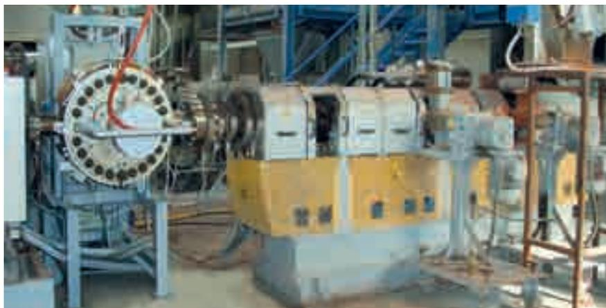
Idealservice is able to produce 20,000 tons of granules and 15,000 tons of SRA (Secondary Reduce Agent), with a recycling rate of almost 90%. It has been able to reach this results also thanks to two Fimic self cleaning filters with a diameter of 500 mm
