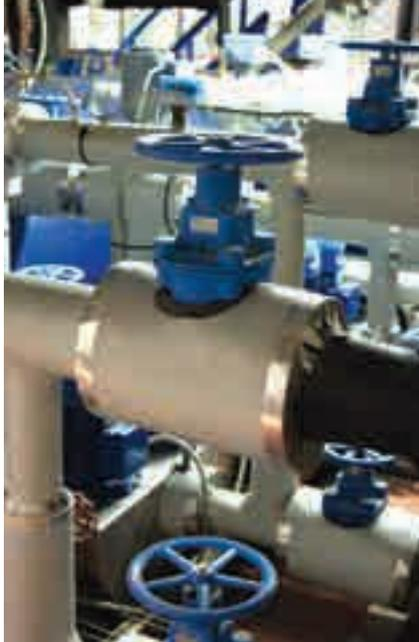
The complex system of pumps, pipes and valves that makes it possible to cool single zones of the extrusion line
