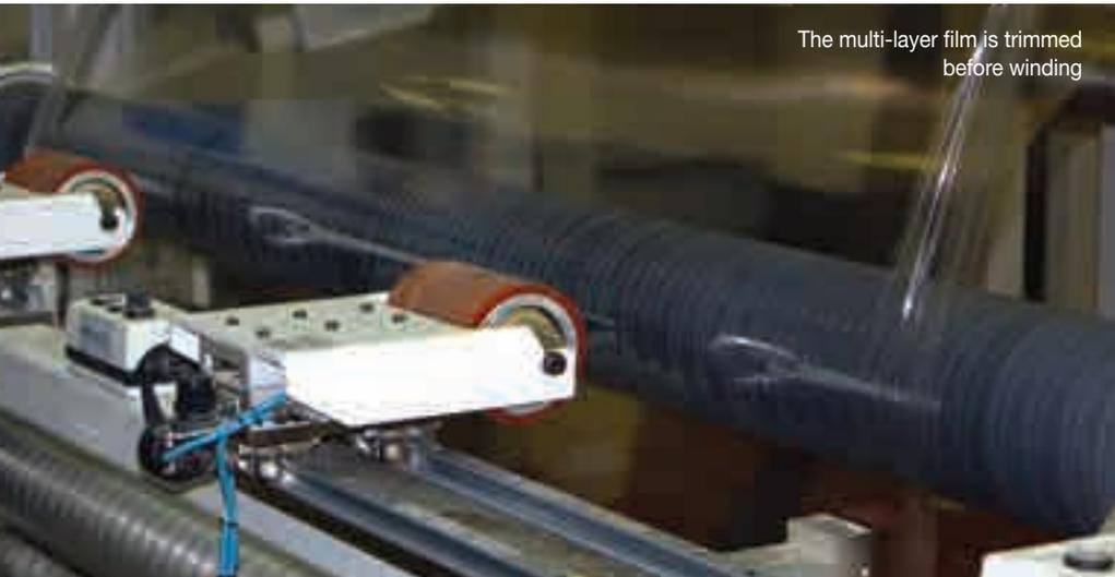
The multi-layer film is trimmed before winding
