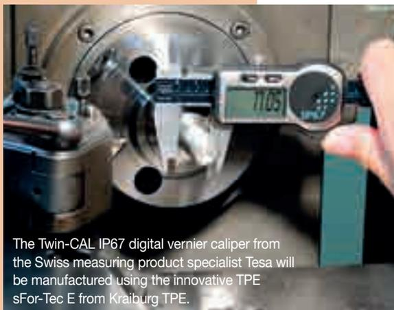
The Twin-CAL IP67 digital vernier caliper from the Swiss measuring product specialist Tesa will be manufactured using the innovative TPE sFor-Tec E from Kraiburg TPE.
