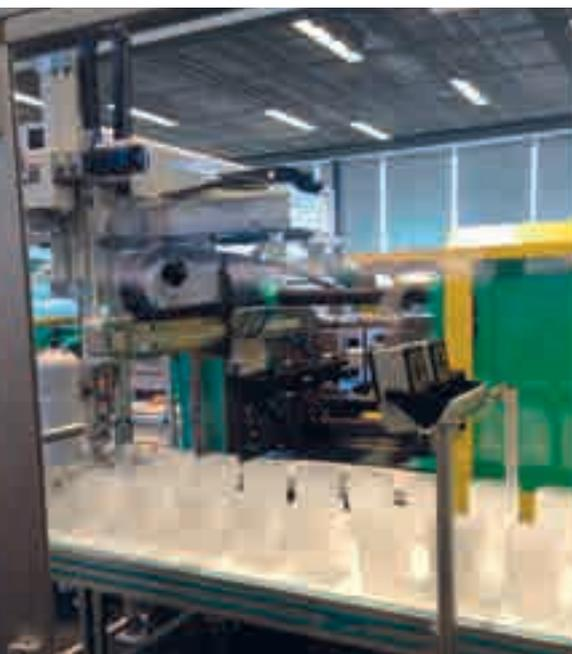
The perfect match among the side entry robot model TZ-1500HM, the 180-ton Arburg Allrounder Hidrive hybrid injection moulding machine and the mould supplied by Hofstetter ensure high output rates and quality in the production of rectangular thin-wall containers
