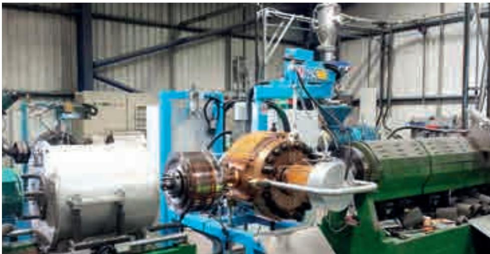
Plasgran has three 400 Fimic filters installed on all of the pelletizing lines. The most recent addition consists in a filter equipped to work in both scraping and backflushing modes, for very fine filtration
