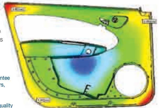
cess, pressure in the part is more even and peaks are reduced, and the part thickness is more uniform. This brings a weight reduction. The holding pressure can be adjusted independently for each nozzle, obtaining more uniform pressure distribution. This minimizes the bending of the mould. Reducing the stress in the mould, also the required stiffness is reduced, allowing steel saving in the tool production.
