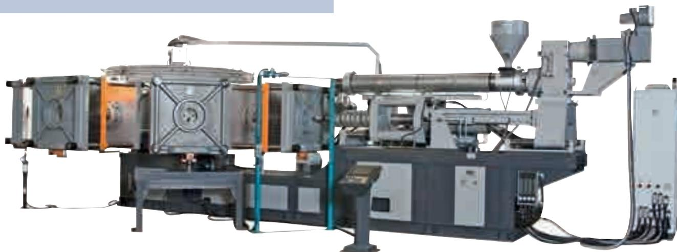
With polypropylene pellets (even recycled) which guarantee efficient feeding and using the new models and 8-cavity moulds, it is possible, to produce bases weighing 150 g (1,200 g of material) at a rate of over 1,200 pieces per hour, which corresponds to a cycle time of under 20 seconds
