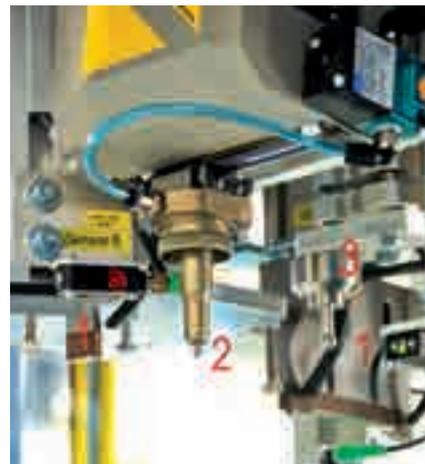
Fig. 1b - Details of function integration: Ultrasonic welding (1), scratch embossing equipment (2), mechanical press-in unit (3) and sensors
