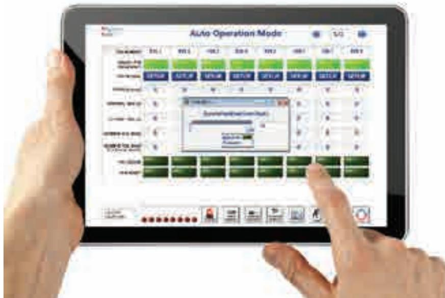
The HRSflow FLEXflow controller grants accurate setting, control and monitoring of the valve pin position, speed, acceleration and stroke.
