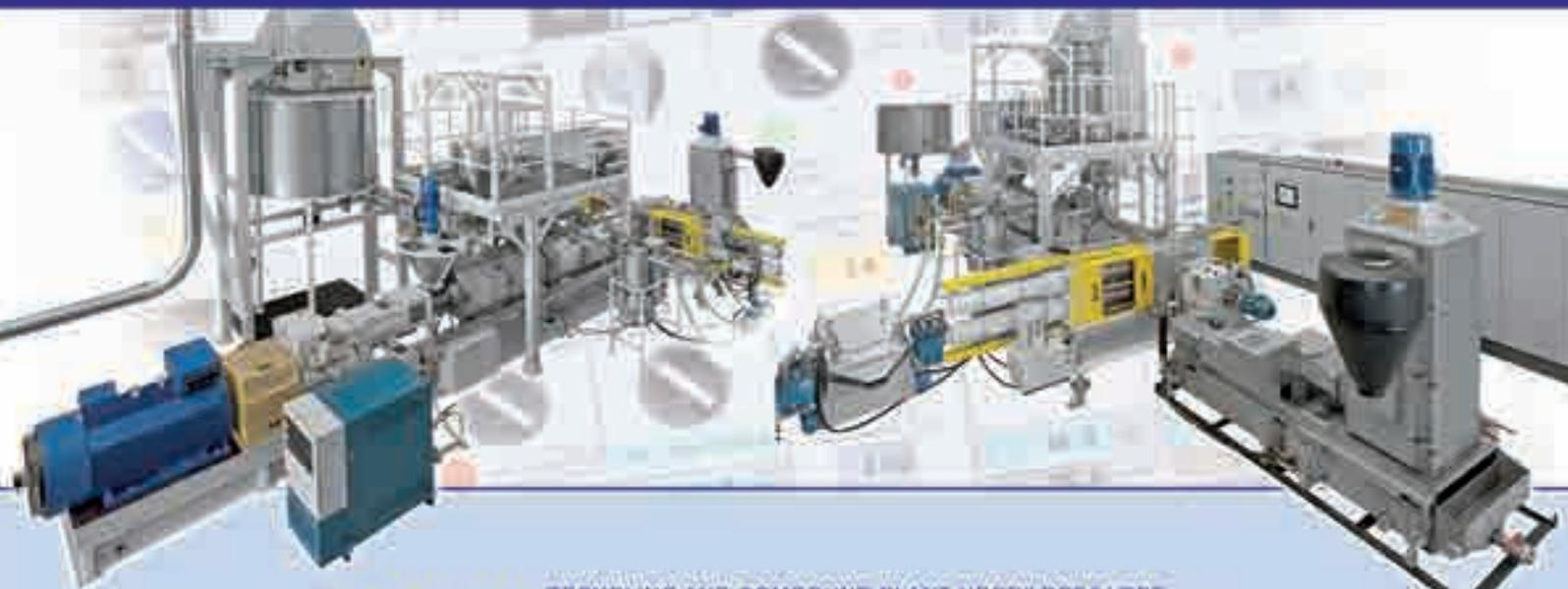
**BiTeCh 110** RECYCLING AND COMPOUND PLANT HDPE/LDPE/LLDPE + CACO<sub>3</sub>, UP TO 50% WITH GRAVIMETRIC DOSING UNIT FOR FILM
