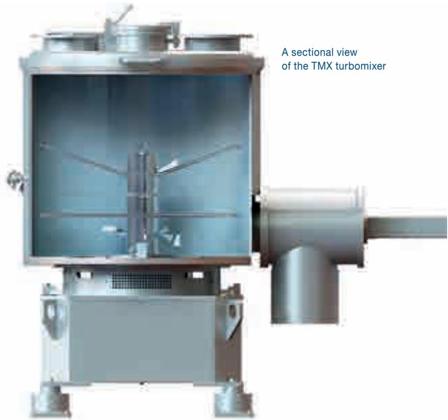
A sectional view of the TMX turbomixer
