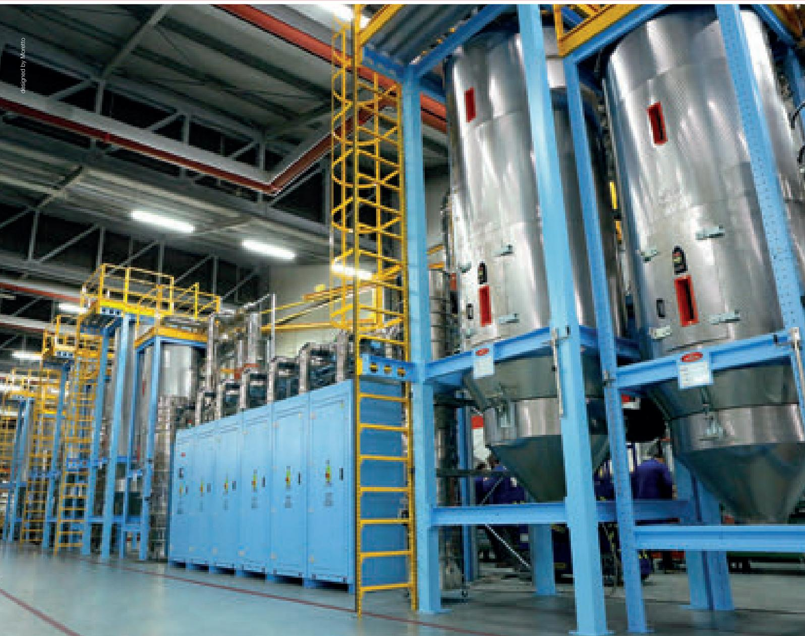
The biggest drying system for plastic materials ever installed in the world, 8,000 kg/h PET.
