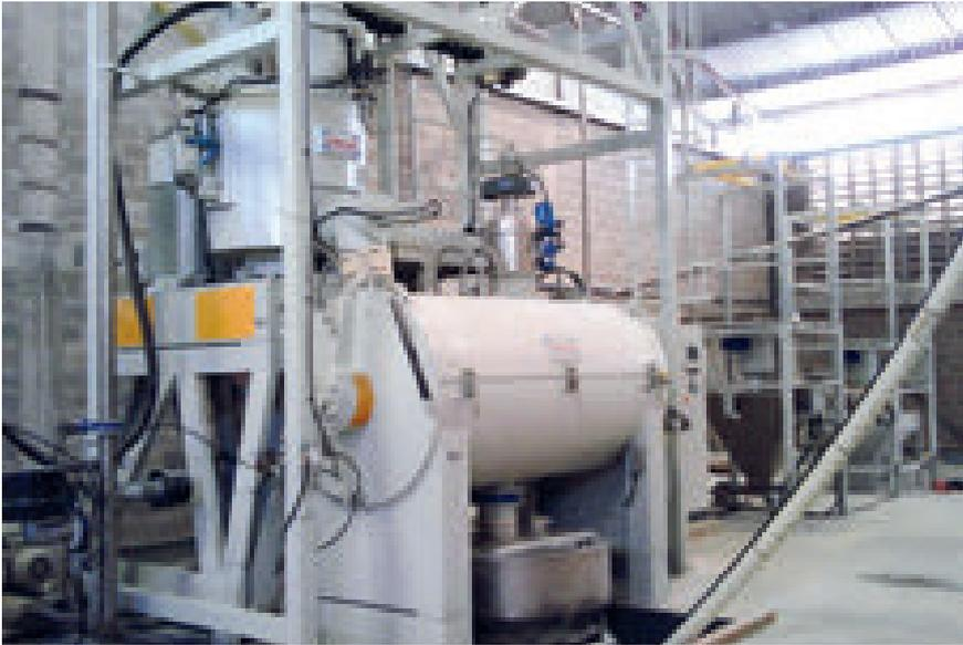
Turbomixer for the preparation of compounds based on virgin or recycled thermoplastic and vegetable materials
