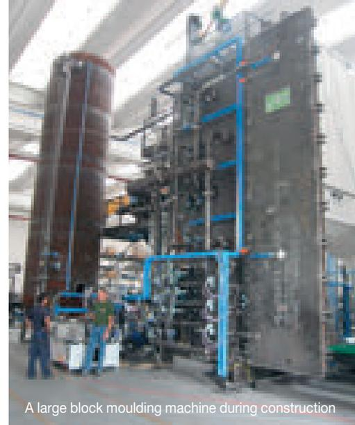
A large block moulding machine during construction
