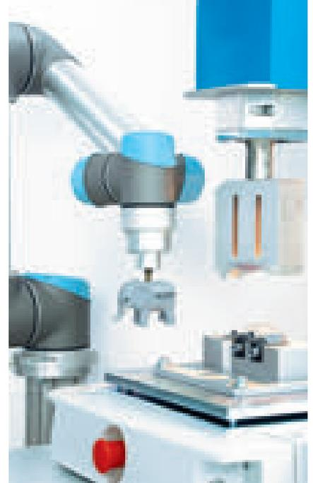
Standard modular ultrasonic welder HiQ Dialog with small-scale robot: handling, testing, welding, and marking of a toy elephant
