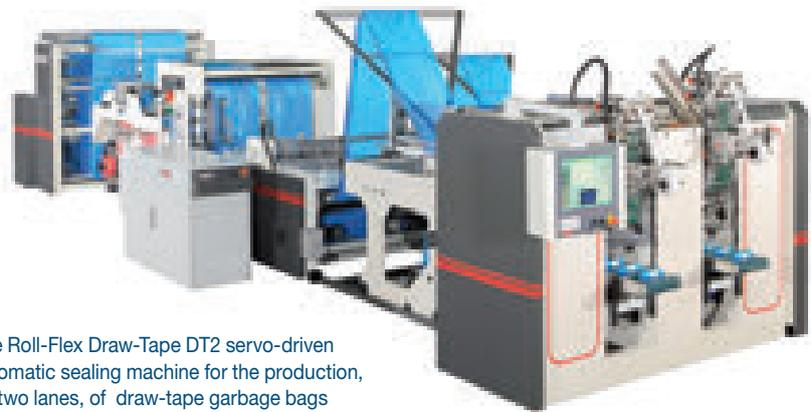
The Roll-Flex Draw-Tape DT2 servo-driven automatic sealing machine for the production, on two lanes, of draw-tape garbage bags
