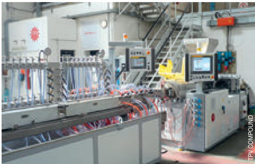
Therefore it is evident that, during the production process, the operator must always know the melt temperature  $T_M$  and the pressure (that depends on  $T_M$ ) at the end of the screw.
