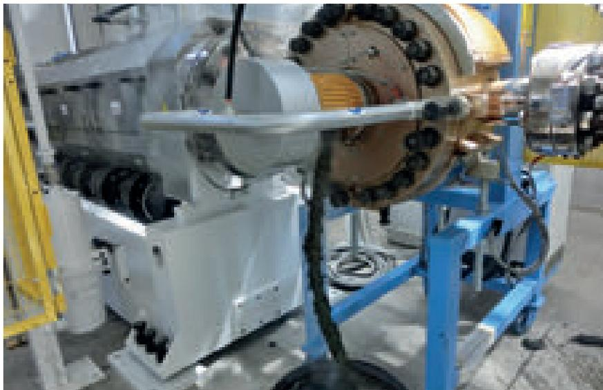
thick. The company can now assure a higher filtration and the resulting material has higher quality. Fimic suggests its customers to purchase a burning oven to clean the screen, which is more expensive than the punched type, so that it can be reused a number of times. The filter does not need specialized personnel to change the screen and the downtime is very short. In 20-30 minutes a new screen is in, also
