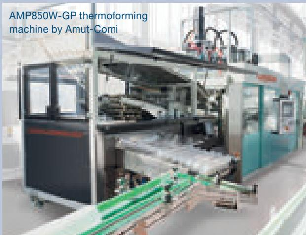
AMP850W-GP thermoforming machine by Amut-Comi
