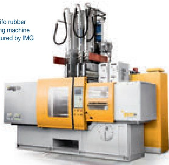
the injection carriage work with a hydraulic system. The machine is also provided with hydraulic core pull integrated. It has a mould for cylindrical drip in HDPE with 24 holes.
