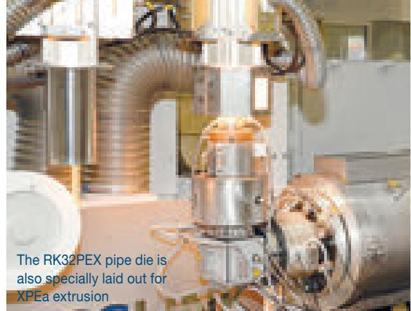
The RK32PEX pipe die is also specially laid out for XPEa extrusion
