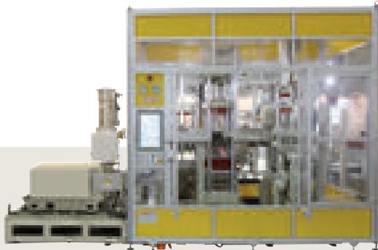
After having been out of the injection stretch blow moulding market for over 10 years, Magic MP is back with the new PET processing BME model, a single-stage 100% electric machine
