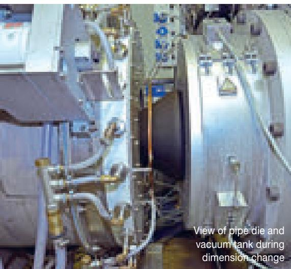
View of pipe die and vacuum tank during dimension change
