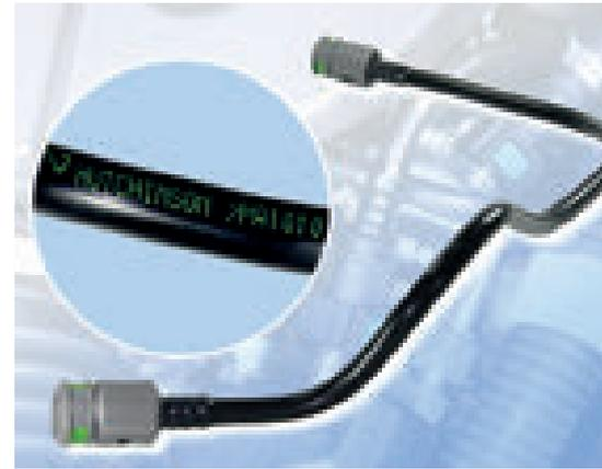
This fuel pipe, used with both diesel and biodiesel fuel, is produced by Hutchinson, in Rivoli (Turin), using Zytel RS PA1010 by DuPont, which is derived from renewable sources. It is installed on several Fiat vehicles featuring turbocharged or multijet engines, e.g. Fiat 500, Panda, Punto, Lancia Delta, Alfa Romeo MiTo, Giulietta
