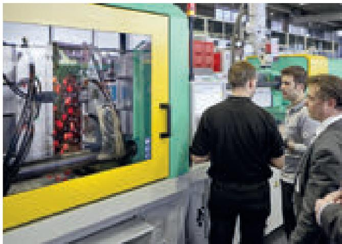
A hybrid Allrounder 720 H in the "Packaging" (P) version equipped with a 72-cavity mould produces so-called PCO-1881 closures for carbonated soft drinks (CSD) in a cycle time of only around 3.5 seconds
