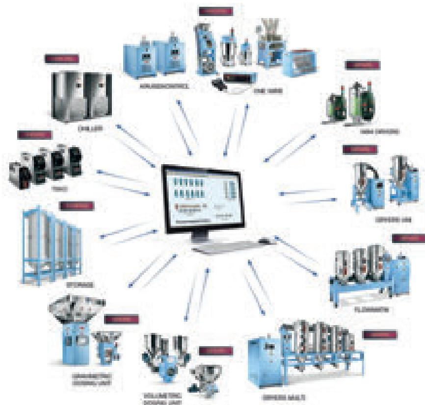
The Moretto Objects Windows Integrated Supervisor (Mowis) is a supervision platform which monitors each single system operation, records all anomalies and creates a chronology in order to set and modify parameters and to generate real-time process reports.
