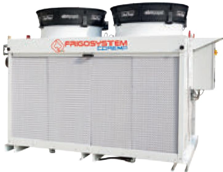
**ADIABATIC HEAT EXCHANGERS** • The new range of industrial process cooling air/water exchangers developed by Frigosystem for industrial process cooling is identified by the initials ACE (Adiabatic Cooling Energy). The adiabatic system permits the exchange of energy between water and air: the energy needed to evaporate the water is taken from the air, the temperature of which reduces as a consequence. The ACE dry coolers therefore use the ambient air to cool process water.
